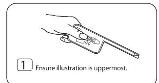
Insert the key all the way into the lock. (Do not turn the key.) This will automatically release the locking mechanism.
