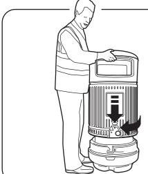
Lift bin body over liner and lower to rest on plinth, turn bin body clockwise to lock.
