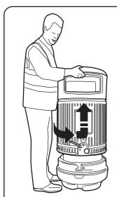
With the key still in position, turn bin body anti-clockwise, and lift bin body over liner.
